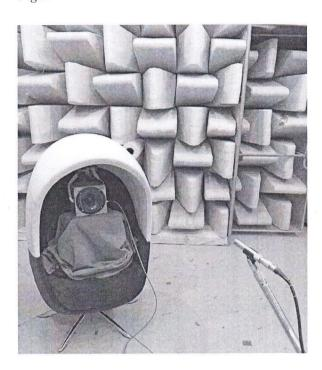
*Picture 2* - 90° *angle between the source and the receiver.*
